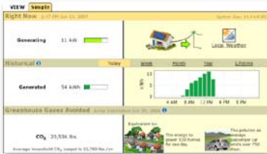
Simple Web view of Basic Residential Monitoring Services showing current and historical power generated along with greenhouse gases avoided. On the right is a link to local weather. Beneath it is a chart showing power generated in kWh by the hour.
